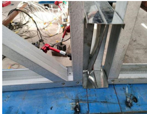
Figure 6. Local buckling failure of I-shaped spliced beams
