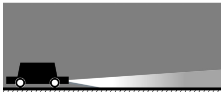
Fig 1. Irradiation range of near-light lamp
