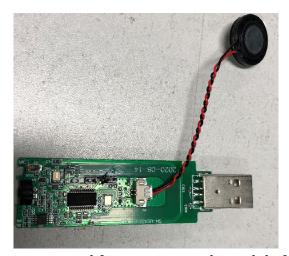
Figure 2. new customized firmware upgrade module for IOT device
