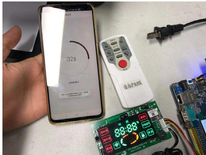
Figure 3. using custom module to help quasi IOT devices pair
