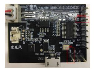
Figure 5. hummingbird m chip and general demo board
